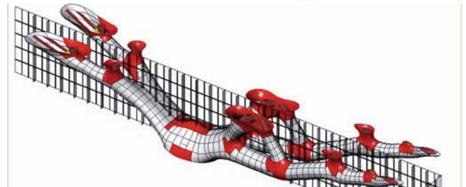
Main canopy support structure - 3 way benned elements (red), while other 75% are only 2 way ( http://www.cgarchitect.com )
