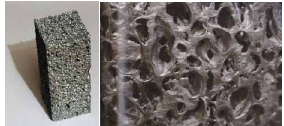
Aluminium casted brick with air spaces made during the hardening process ( "Matter" / Gail Peter Borden)
