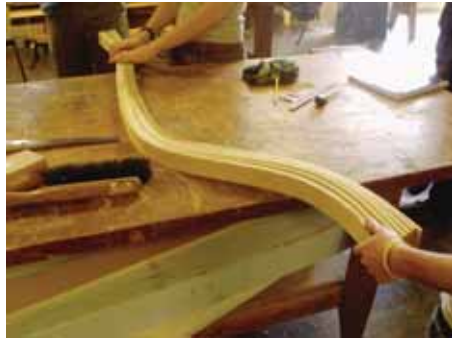
Bent wood laminations before glue up. http://ocw.mit.edu/ans7870/4/4.296/s05/lecturenotes/gallery2/8.html
