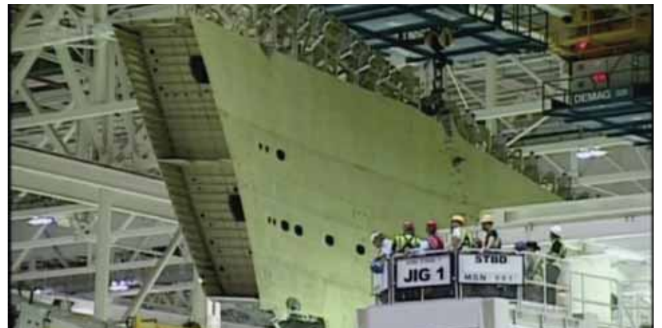
Before covering, all the systems are being intalled. the accuracy is reached by laser measures
