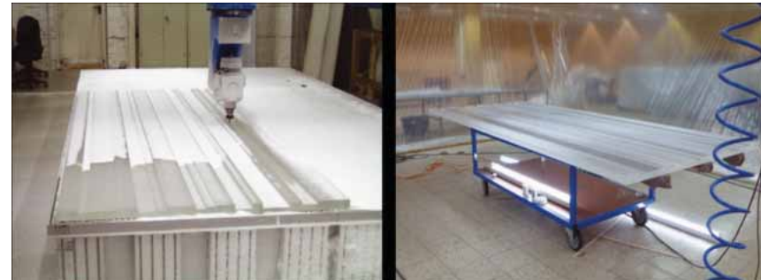
Reiss London. Acrylic milling process and finished facade panel.
