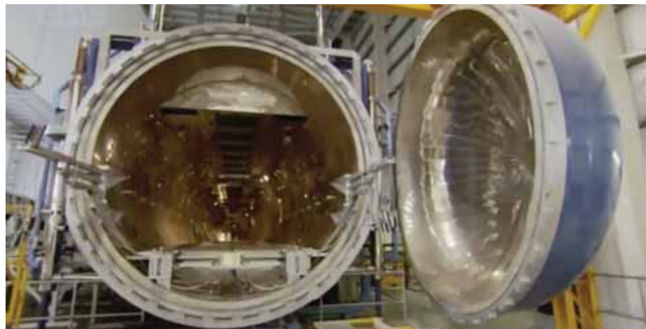
The shaped sheet is rolled with a nylon in vacuum and baked in the oven for 24 H in 180 degrees
