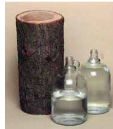
Fresh wood has high moisture content. This log of Eastern hemlock contains almost 6 litres of water. Completely dry, the log would weigh one-half as much as its green weight. (Arno, 1993)
