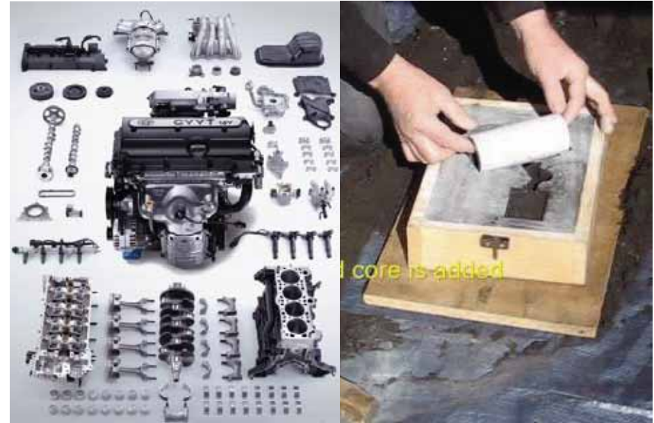
Engine parts in different shapes and sizes manufactured mainly from metals. Casting in a sand core form. ( http://www.tradekorea.com )
