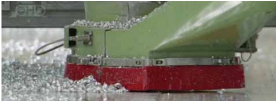
The sheet is polished according to CAD file and loses 75% of material (from 5 to 1 ton)
