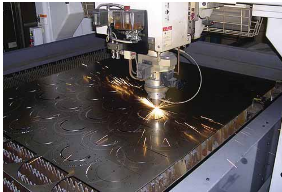
Laser Stamping by laser beam ( http://www.power-technology.com )
