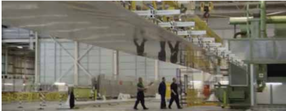
Aluminium Sheets 42X6 m transferred to te CNC machine
